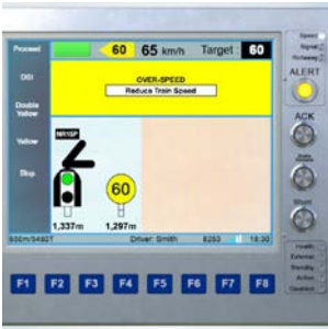
EN4CER:4MTU Driver Advisory System and automatic train protection
